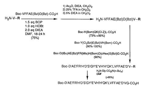
Fig. 2. Synthesis of protected  $\beta AP$  (1–25).
