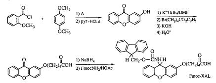
Fig. 1. Preparation of Fmoc-XAL handle.
