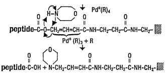
Fig. 1. HYCRAM<sup>TM</sup> release technology in SPPS.
