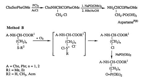
Fig. 1. Conversion of some amino acid side chains into phosphonate groups.
