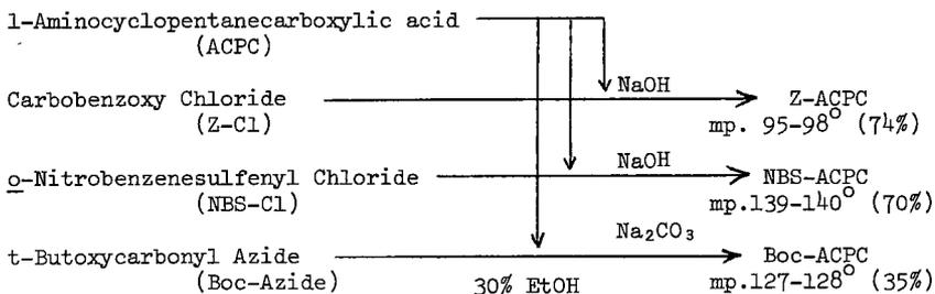
FIGURE 3: Synthesis of N-ACPC Protected Derivatives.
