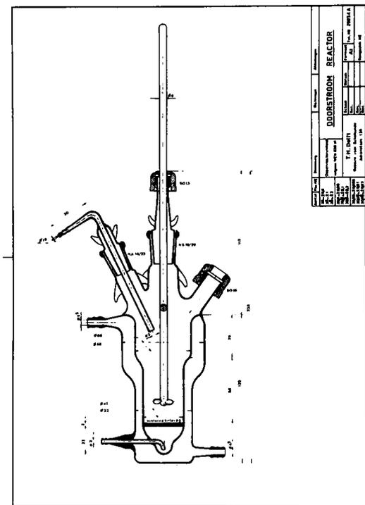
Full-flow reactor for kinetic measurements.
