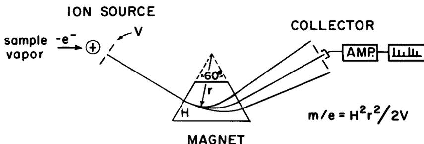
Figure 1. Schematic of a Low Resolution Mass Spectrometer
