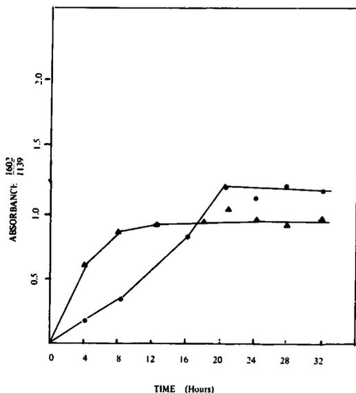
Fig. IV. Time study of oxidation of sulfide support (MTP) to activated sulfone (MSP) support. 30%  $H_2O_2$  in HOAc (4:6); 4 equivs of *m*-chloroperbenzoic acid in dioxane.
