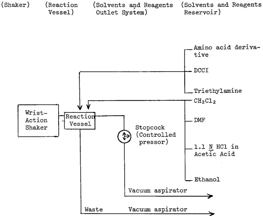
**FIGURE 1:** System of Non-Automatic Manual Valving Apparatus for Solid-Phase Peptide Synthesis.
