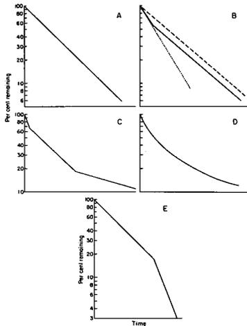
Fig. 6. Typical thin film dialysis escape plots. A = a single solute behaving ideally, B = a mixture of two diffusional sizes ..... and --- whose sum gives —, C = a mixture of three diffusional sizes, D = a mixture of several diffusional sizes or a solute behaving nonideally, E = a solute showing self-association
