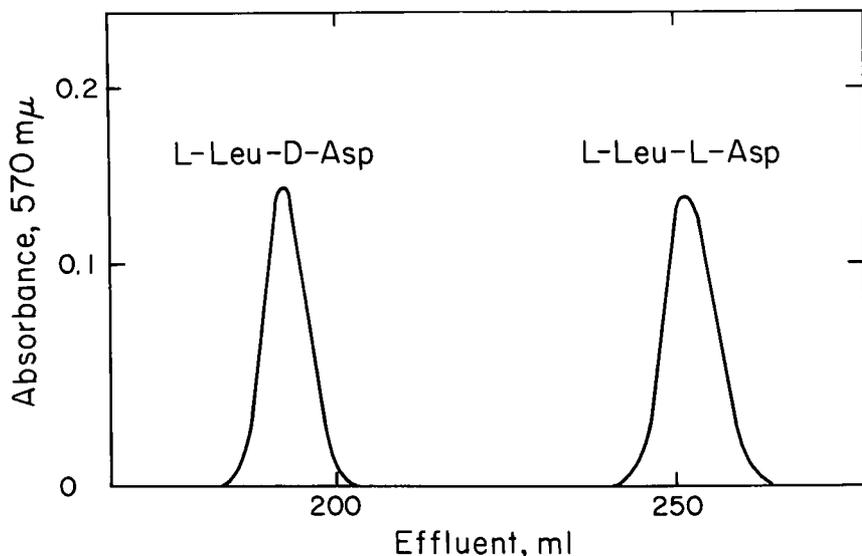
Fig. 2 - Separation of L-Leu-D-Asp and L-Leu-L-Asp on the amino acid analyzer at pH 3.25, 52°. A 0.9 x 62 cm column packed with Spinco AA-15 resin was used.
