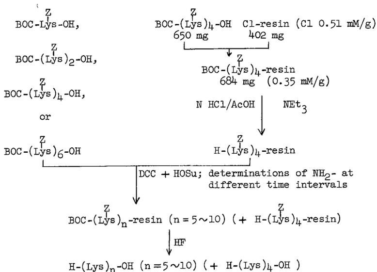
Fig. 2. Condensation of BOC-peptide acid in different sizes and a peptidyl-resin.
