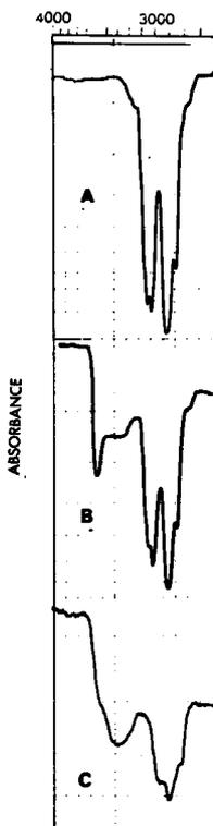
Fig. II. Infrared spectra of chloromethyl polymer (A), Phenol-Sulfide Polymer (B), Resitol Type-MTP polymer (C).
